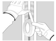
Apply thoroughly mixed Sikadur®-Combiflex® Adhesive, Sikadur®-31 CF or Sikadur®-31 DW on both sides of the joint / crack onto the prepared substrate, using a suitable trowel. If the concrete substrate is damp, force the adhesive well into the substrate. Layer thickness of adhesive should be 1 - 2 mm and the width on each side at least 40 mm.
